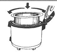
Place the inner lid to the outer lid by pressing the inner lid to cover over the inner lid shaft.
