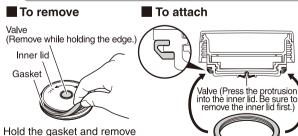
After pressing the valve, check that the protrusion has come out from the other side.
