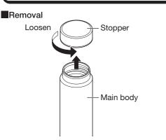
Turn the stopper counterclockwise to remove it from the main body.
