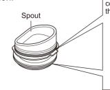
Upper stopper gasket Convex section -Attach the stopper gasket so that the convex section of the gasket comes out.
