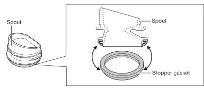
Slowly remove the stopper gasket while holding its edge. When attaching the stopper gasket, make sure to fit it completely in the proper direction.
