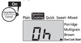
If a longer cooking time is required, you can set the disired additional cooking time. Press the [Hour] and [Min] keys to set the additional cooking time with the Keep Warm lamp turn on. The cooking time can be extended up to 30 minutes. a maximum of 3 times.
