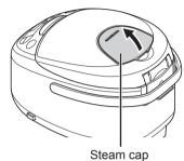
Turn the inside portion of the assembly as shown in the illustration to loosen it.
