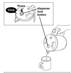
After the hot water has been dispensed, be sure to press the dispense lock button to set it to the "locked" status.
